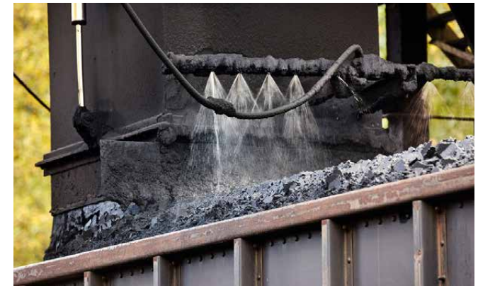
Coal wagon profiling and veneering at Buchanan mine
